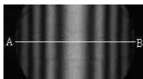
Fig. 1a - (200) CBED dark field disk.
