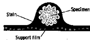
Fig. II.39. Schematic representation of a specimen particle completely embedded in a negative stain. (From Hayat and Miller, p.2)
