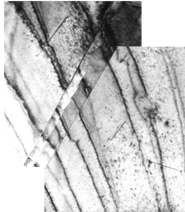
Ni - 6Al - 6 Si 3 MeV Nickel Ion Irradiation- 3 dpa
